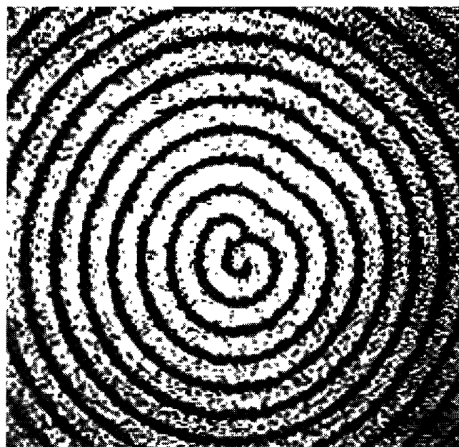
Figure 10 Intensity difference images of a target pattern with a broken spiral centre 132 min after mixing the reagents, produced from two images collected at 440 nm and 10.0 s apart. The dark bands represent the distance that the wave has travelled between image shots. Image size 19.3 \times 19.3 mm. Experimental conditions: [\text{KBrO}_3] = 0.3 \text{ mol l}^{-1} , [\text{H}_2\text{SO}_4] = 0.25 \text{ mol l}^{-1} , [\text{CH}_2(\text{COOH})_2] = 2.5 \times 10^{-2} \text{ mol l}^{-1} , 1.0 \times 10^{-5} \text{ mol g}^{-1} immobilised on > 400 mesh size Bio-Rad Analytical Grade 50W-X4 cation exchange resin. (Reproduced with permission from Maselko et al. 28 © 1989 The American Chemical Society)
