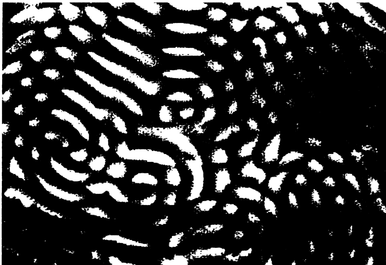
Figure 11 Chemical waves propagating on the surface of a ferroin-loaded Nafion membrane suspended in a cstr pumped with BZ reaction mixture. Image shows the intensity of light transmitted through a membrane 0.18 mm in thickness, 4.5 h after initiation, residence time of 56.93 min; field of view is 6.3 \times 4.7 mm. Nafion loading 38.7%. Reactant concentrations ( \text{mol l}^{-1} ) in cstr: [\text{NaBrO}_3] = 0.19 , [\text{H}_2\text{SO}_4] = 0.24 , [\text{CH}_2(\text{COOH})_2] = 1.9 \times 10^{-2} , [\text{ferroin}] = 5.8 \times 10^{-5} , [\text{KBr}] = 8.7 \times 10^{-4} temperature 25.0^\circ\text{C} (Reproduced with permission from Winston et al. 29 © 1991 Macmillan Magazines Ltd)
